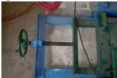
Fig. 14 SLIDING ARRANGEMENT OF MOTOR
